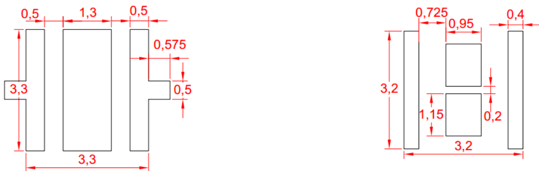
Fig 26. Recommended Solder Pad (推荐焊盘)
